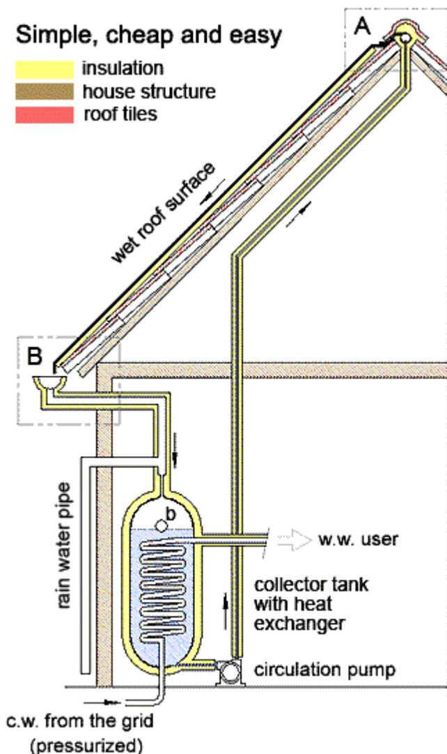
Hence, all you have to do is to provide a flat and underneath insulated surface on the roof of the house and spray water over it, not more than to keep its surface wet all over. For this you would need a specially prepared feed water distribution pipe (view A), lying along on top of the roof - any mechanical workshop can make that on order.
