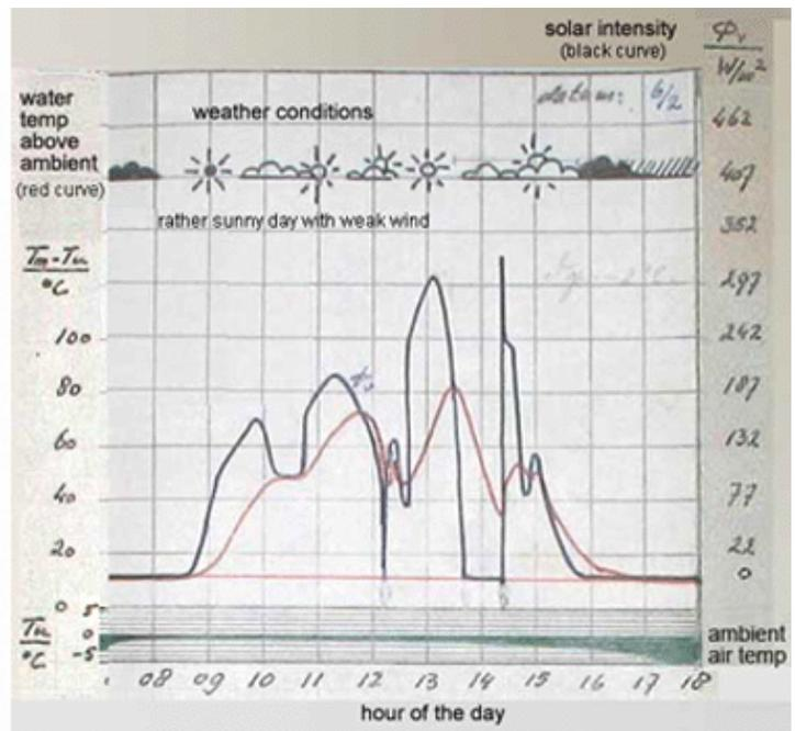
The "secret" simply is to know that plain water is a black-body absorber for infra-red (heat) radiation, fortunately having its peak sensitivity on the same wave lengths (1.95, 3 and 6  $\mu m$ ) that the atmosphere allows radiation from the sun to reach Earth's surface. Just as fortunately, common window glass is fully transparent for those wave lengths.
