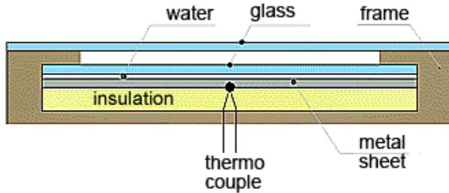
Just an insulating sheet of polystyrene, a metal and a glass sheet on top, with around 0.5 mm of water in between, a thermo couple soldered on the metal sheet to measure the temperature, a sealing frame around with a second glass sheet and that was it.
