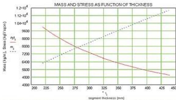
From the curves above we see that for given diameter, number of segments and diving depth, the mass weight of the shell is proportional and the allowed tensile surface stress inversely proportional with the thickness (height) of the segments.
