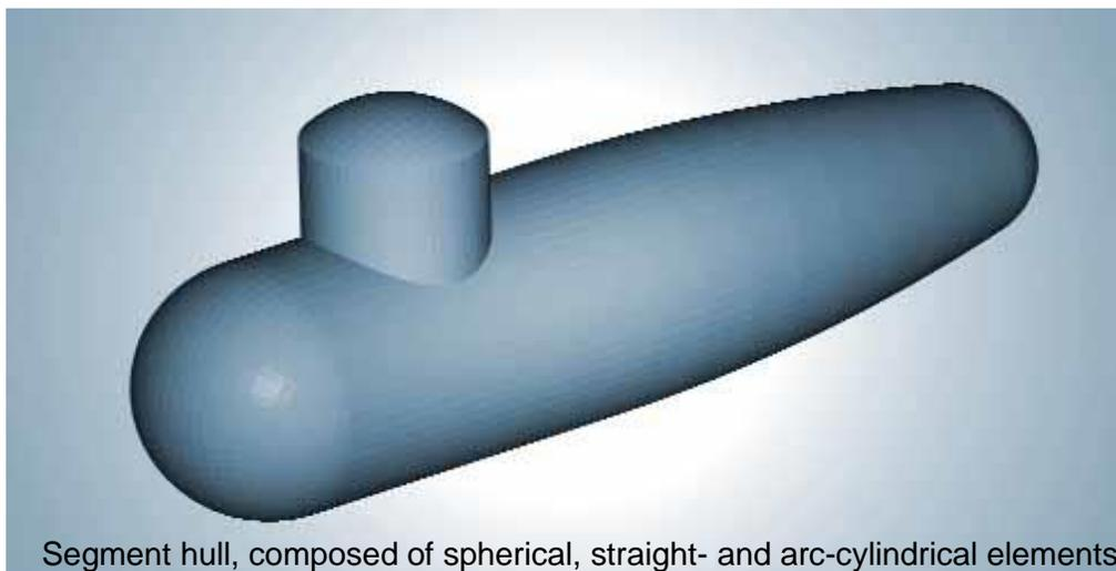
Segment hull, composed of spherical, straight- and arc-cylindrical elements
