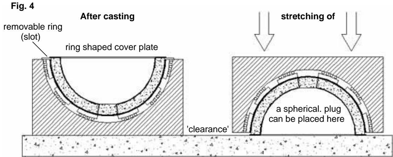
As the material is stretched 2-dimensionally it will likely become necessary to do it in warm condition so that the shell will shrink around the segments as it cools down. Before this happens, the joint between the cover plate and the outer shell is welded, whilst the outer shell is still pressed down towards the joint. I am aware that this is a very rough description and that many details remain to be solved, but this has to be done by experts who can do that better than I.
