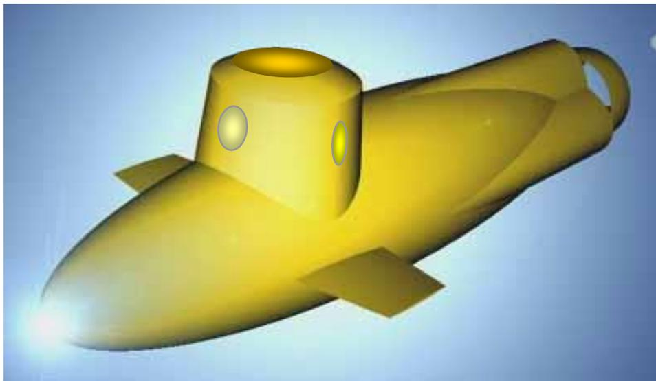
Segmented hull: elliptical longitudinally, circular transversally
